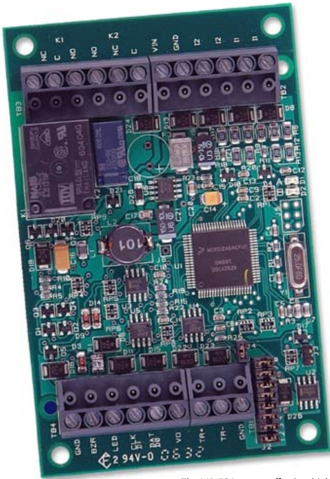
The MR-50 is a cost-effective, high-performance single reader I/O module.
