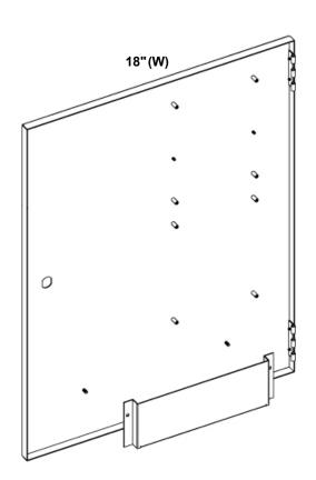
Door is shown separately only to provide detail. Door is not removable.
